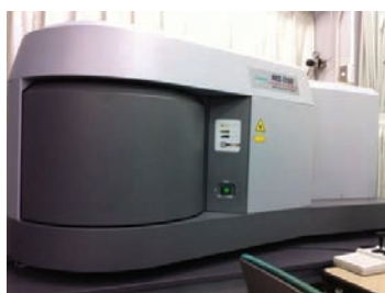
NRS-7200 with low wavenumber measurement unit
