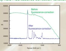
Spectra Manager II for the NRS-5000/7000 offers revolutionary features to simplify previously difficult measurement and analysis tasks, while adding various user-support tools such as auto-fluorescence-correction, wavenumber correction, intensity correction, and a novel user-advice function. With a graphical user interface, the Raman microscope analysis program offers maximum ease of use for microscopic measurements.
