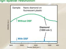
Unique DFS function provides higher spatial resolution than normal confocal optics to irradiate only the target sample.
