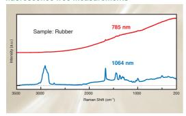
All models can integrate Near-IR excitation lasers, especially useful for samples which generate fluorescence, even when excited using 785 nm.
