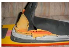
Figure 1: Digital image of a degraded neoprene wrap on a 1976 EP X2 slalom waterski.
