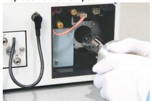
Replacement of D<sub>2</sub> and halogen lamps can be performed from front panel.
