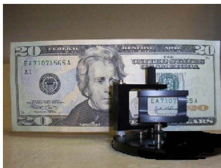
Figure 1. Solid sample holder accessory FPA-810 with $20.00 bill.
