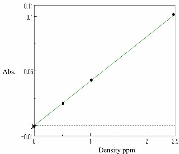
Fig. 3 H<sub>2</sub>O calibration curve
