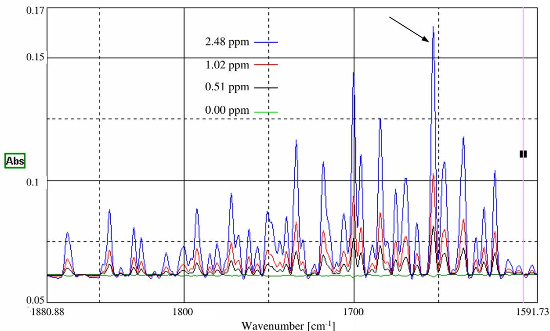
Fig. 2 Expanded region for spectra of low concentration H<sub>2</sub>O
