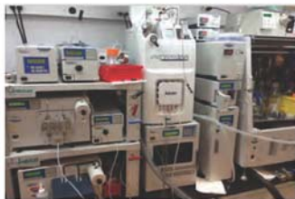
JASCO Preparative SFC system with fraction collection and Advion expression CMS
