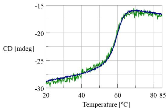
**Figure 2.** Thermal denaturation curve of ribonuclease A measured at a wavelength of 222 nm. The green curve was obtained using the capillary cell while the blue curve was measured using the 1 mm rectangular cell.
