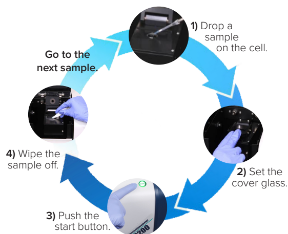
Figure 1. Flow chart illustrating the sample preparation procedure using the One Drop accessory.
