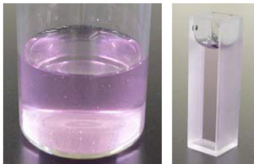
Figure 2. Screw samples after the chromogenic agent was added to the extraction solutions and pre- (left) filtration and post (right) filtration of the solutions.
